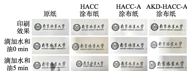
图 20 不同涂布纸的印刷效果以及印刷后防水防油效果 Fig. 20 Printing effect of different coated papers and waterproof and oil-proof effect after printing
